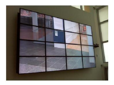
Assuming that 1080p flat-panels are used to build the wall, this creates a total resolution of 7680x4320. Rather than stretch a low-res image to fill this resolution, we're going to use the AV Binloop HD to provide 16 individual 1080p sources to feed the wall with native resolution content. Furthermore, we are going to add flexibility to the system by adding a V16Pro show controller and some of our ShowTouch panels.
